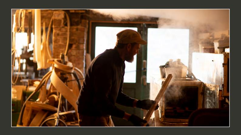
A piece of steam-hot wood being pressed into a curve. A sliver of time when it can be sensitively coaxed into shape before it cools and sets.
